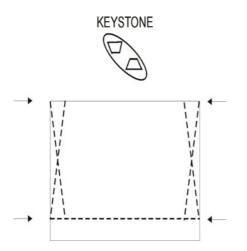
To adjust image vertically and make a square image. Adjust the keystone function by pressing the keystone button on the remote control or through OSD menus.
